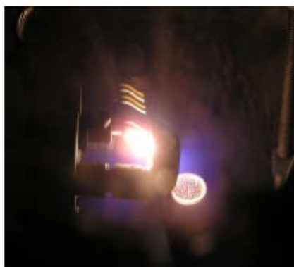
Fig. 3. Photo of the GTVA plasma ignited in methane.
