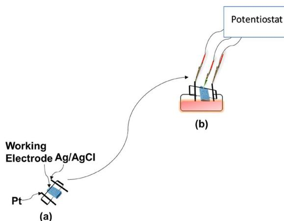
**Figure 3.** Schematic representation of the (a) disposable sensor and (b) setup of the measurement.
