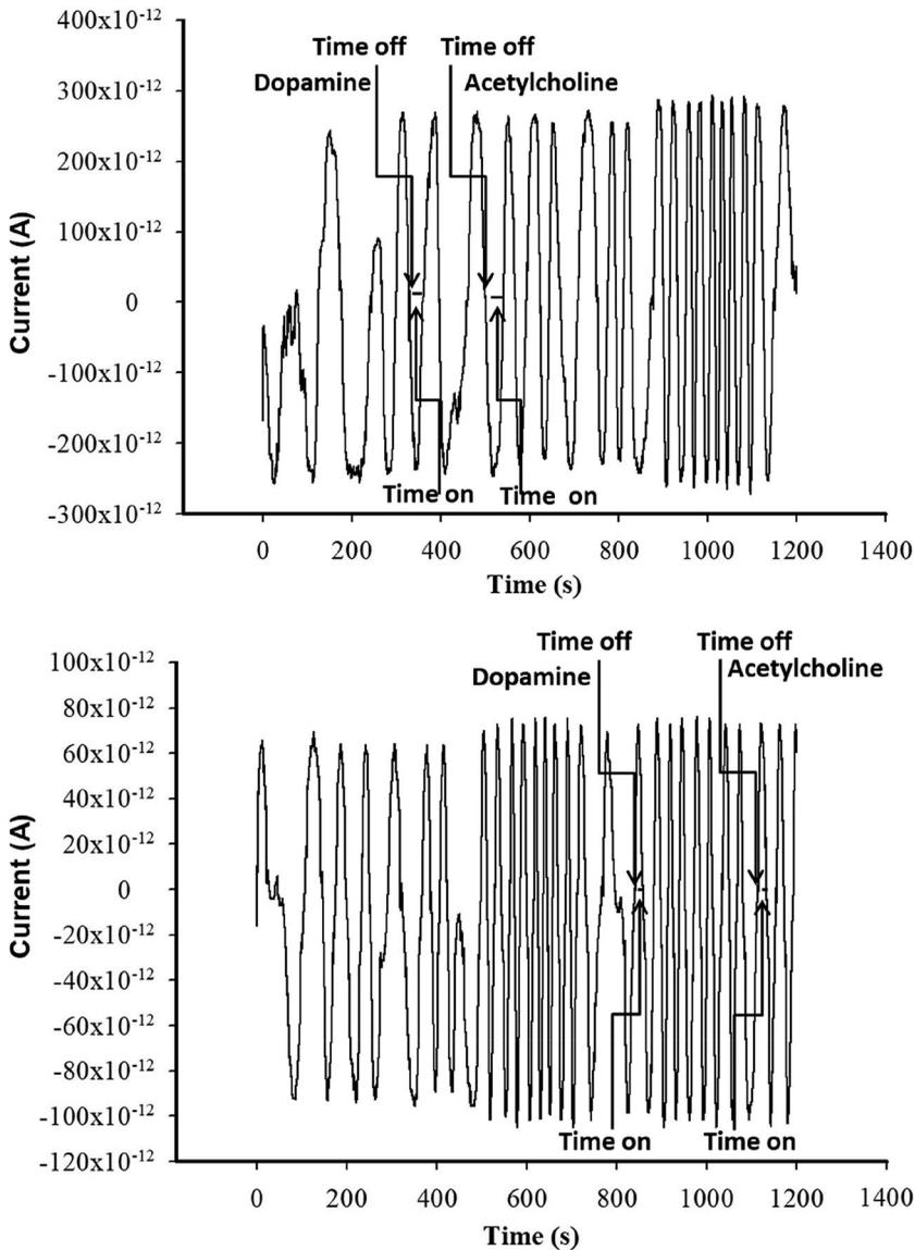
**Figure 2.** Diagrams obtained for the screening of whole blood using the sensors based on (a) Maltodextrin I, and (b) Maltodextrin II.
