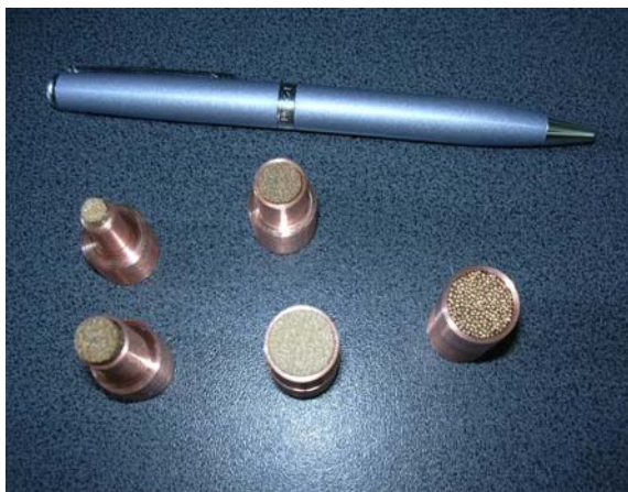
Fig. 2. Different types of the disk of filter (powder of brass) after encapsulation.
